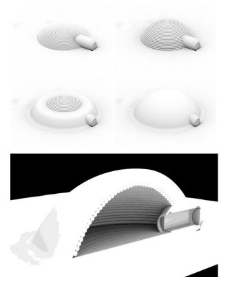
Fig. 2: Building the wall using a temporary inflatable support. Sequence: left to right and top to bottom.
