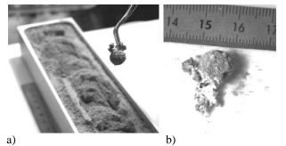
Fig. 8: a) Sample #6 being extracted from the regolith simulant container after the test. b) Size of sample.
