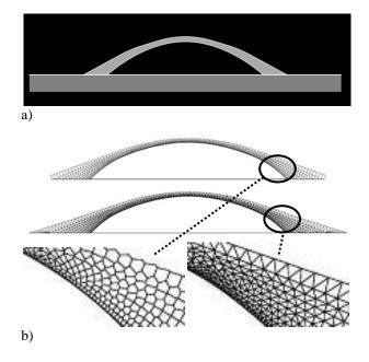
Fig. 3: a) Wall profile obtained by enveloping regolith slope, radiation, and micrometeoroids requirements.b) Optimization of structural elements.
