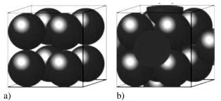
Fig. 6: a) Simple Cubic Packing. Void/full ratio = 48%.b) Cubic Close Packing. Void/full ratio = 36%.
