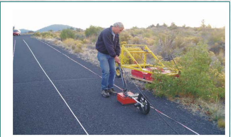
Figure 7 – GPR data collection at Hercules with the 400 MHz antenna and survey wheel
